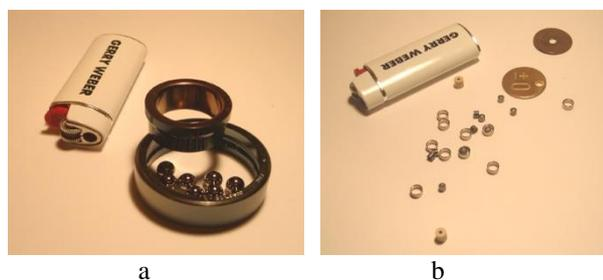
Figure 1 Appearance of some machine parts with monocrystalline carbon coating: a– ball bearing (disassembled), b - micro-bearing.
