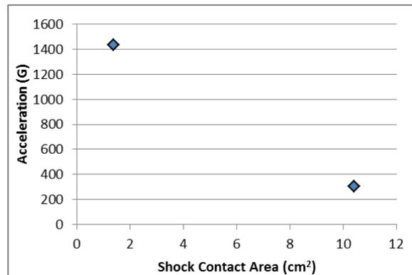
Figure 5 Relationship between Shock Contact Area and the amplitude of Shock Acceleration (At drop height 29.5cm, and damper thickness 2mm).
