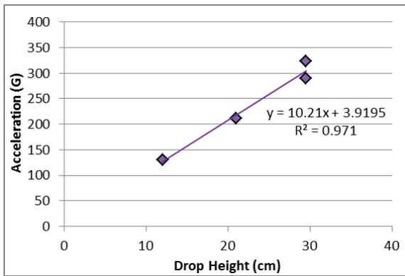
Figure 3 Relationship between drop height and the amplitude of shock acceleration (At damper thickness 2.0mm, and contact area 10.4cm<sup>2</sup>).
