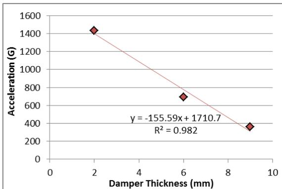
Figure 4 Relationship between Damper Thickness and the amplitude of Shock Acceleration (At drop height 29.5cm, and contact area 1.4cm<sup>2</sup>).
