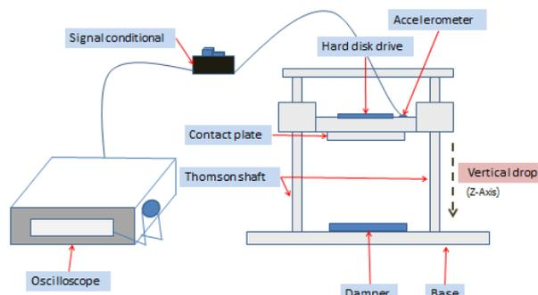
Figure 2 Overview of simple shock tester.
