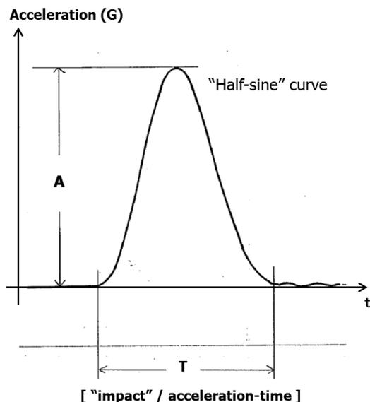
Figure 1 Desired Half-Sine wave shock output.
