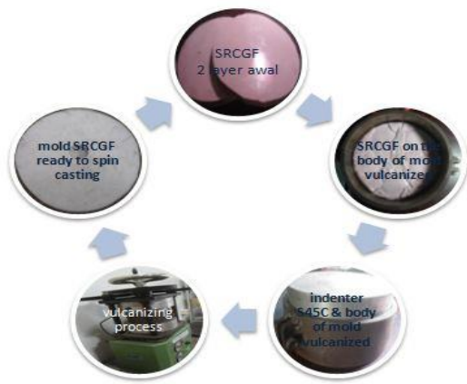
Figure 2 Vulcanizing SRCGF material process steps in a metal souvenir industry.
