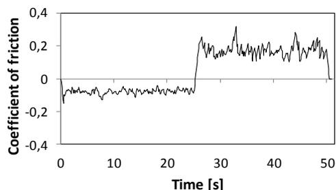
Figure 2 Coefficient of friction for one cycle at a normal load of 9 mN and a crossing angle of 90°
