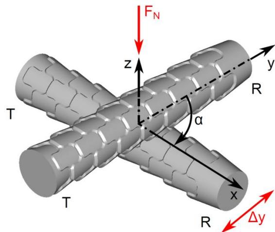
Figure 1 Crossed fibres test arrangement
