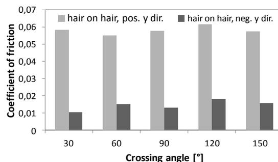
Figure 4 Coefficient of friction for different crossing angles and a constant normal load of 9 mN
