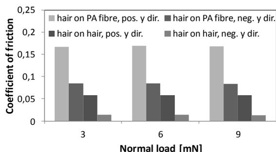
Figure 3 Coefficient of friction for different normal loads and a crossing angle of 90°
