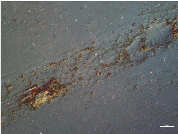
Figure 4 Worn surface of worn \text{Si}_3\text{N}_4 ball – bright field DIC, 10 \mu\text{m} scale (10x100).
