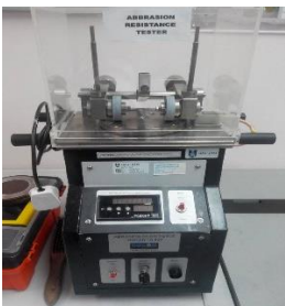
Figure 1 Abrasion Resistance Tester and the schematic diagram
