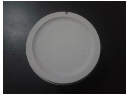
Figure 1 Actual plasma sprayed Mullite coated piston crown.
