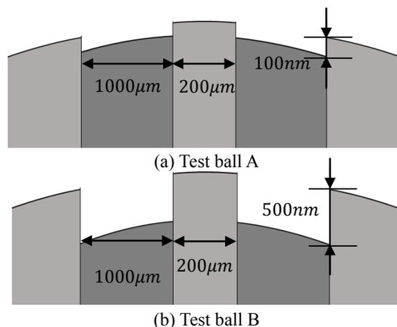
Figure 2 Illustrations of the test balls with downsteps.
