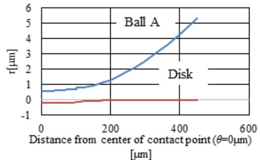
Figure 5 Deformation of disk and ball for pressure distribution calculated using the Reynolds equation.
