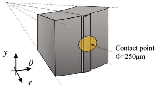
Figure 4 Analytical model for FEM analysis.
