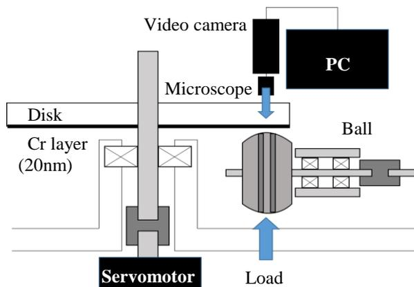
Figure 1 Disk-on-ball friction tester with optical interferometry.
