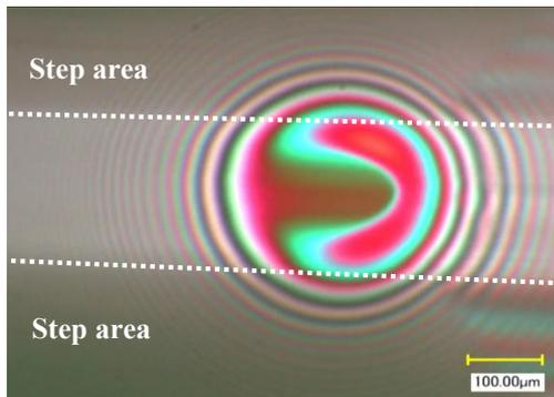
Figure 4 EHL film shape for test ball A at rotational speed of 1.5 m/s.
