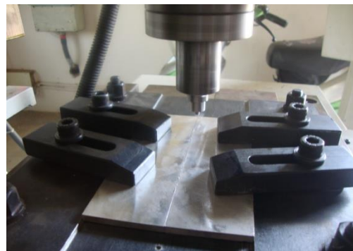
Figure 1 Arrangement of AZ80A Mg Alloy plates along with the with taper cylindrical pin profiled tool.
