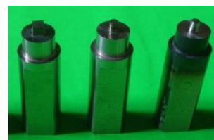
Figure 2 HSS tools with straight square, straight cylindrical & taper cylindrical pin profiles.
