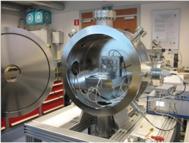
Figure 3 Fiber holder mounted in a vacuum chamber.
